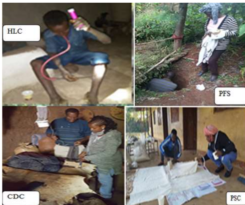
Figure 2: Human landing catches (HLC), Pyrethrum spray sheet (PSC) pit shelter (ps), CDC Light Traps (CDC), 2016-2017
